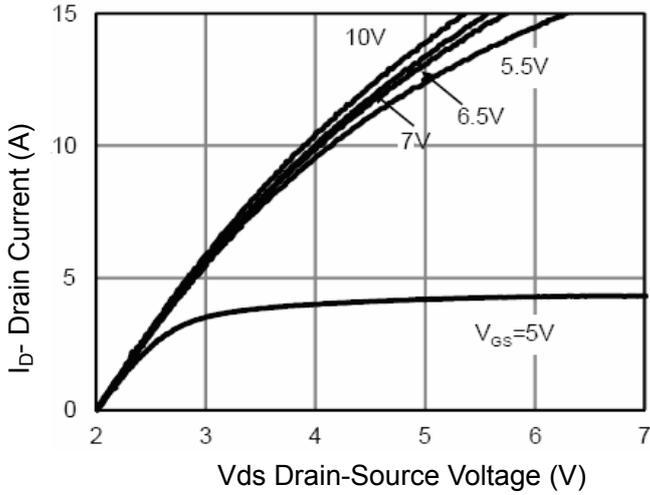
Figure 1 Output Characteristics
