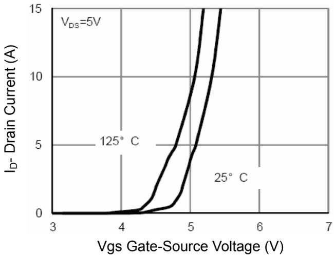
Figure 2 Transfer Characteristics
